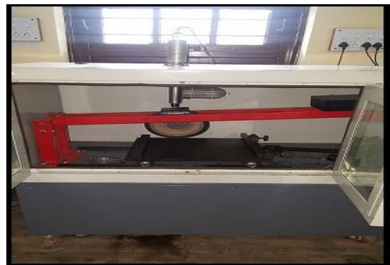
Fig. 4 Wheel Rut Shaper
